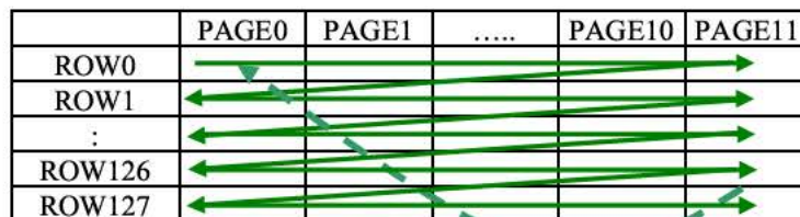
Figure 0-7 : Address Pointer Movement of COM-Page H-mode
